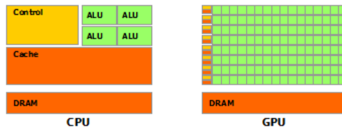
Figure 2. The GPU devotes more transistors to data processing (image taken from CUDA programming guide) [2]
